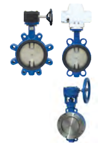
VTM Resilient Seated Butterfly Valves 32mm to 1000mm; Lever / Gear / Motorised Cast Iron / Ductile Iron / Cast Steel; PN10/16/25
