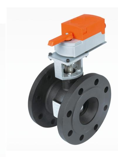
Electric ball valve assembled force of actuator from 16Nm, 24Nm, to 32Nm with DN65--DN150 valve body. Supply voltage optional: AC24V±10% 50/60Hz or AC220V±10% 50/60Hz, 0-10VDC or 4-20mA control signal can choose, as well as 0-10VDC position feedback signal. It widely used in air conditioning, refrigeration, heating and building auto control system, can adjust the medium flow precision, achieved goal to control temperature, humidity, pressure and energy saving.
